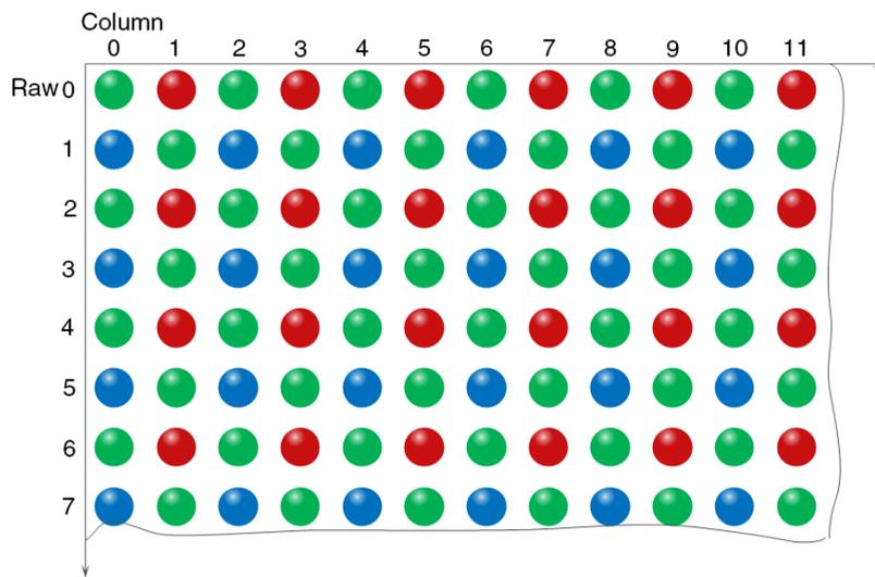
When the pixel format is set to BayerGR8, the value of each pixel in the output image of the camera is 8 bits. According to the location difference, the three components of red, green and blue are respectively represented. The format in the memory is as follows:
