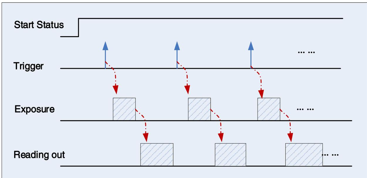
Figure 8-7 Trigger acquisition process
