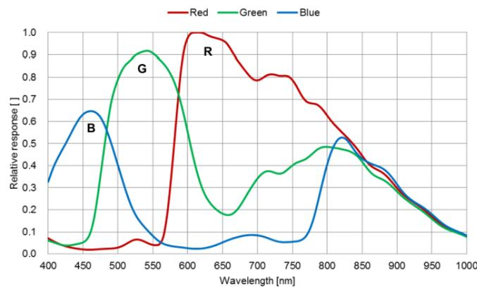
Figure 4-1 MARS-1231-46G5C-P sensor spectral response
