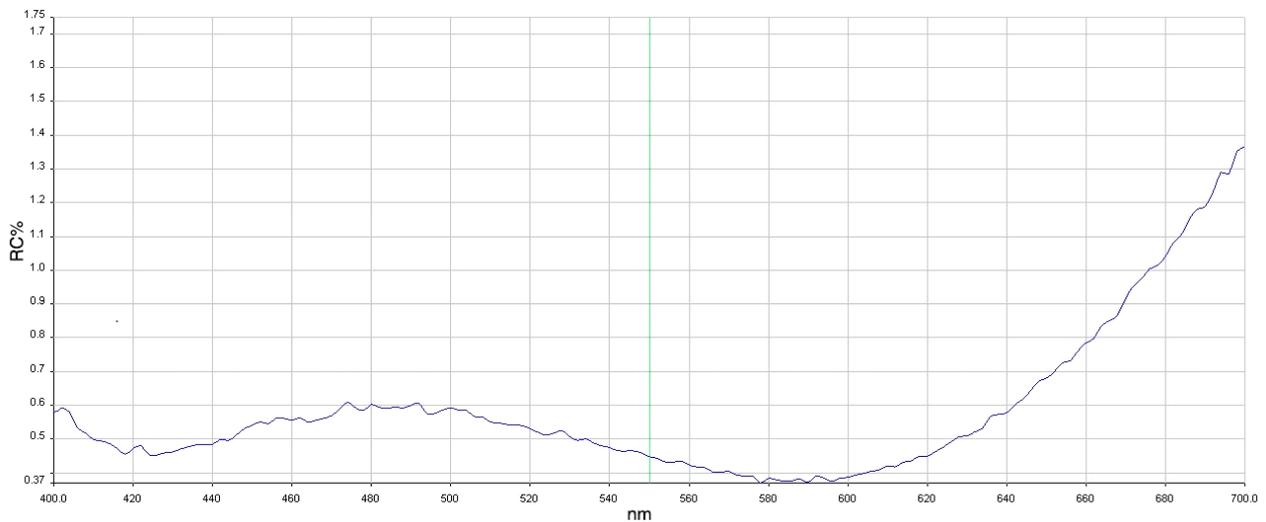
Figure 6-2 Transparent glass reflectance curve for MARS series mono camera
