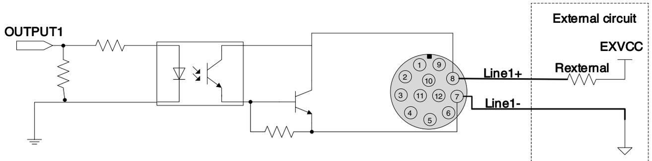
Figure 7-5 Opto-isolated output circuit
