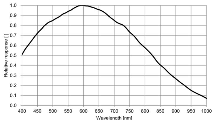
Figure 4-2 MARS-1231-46G5M-P sensor spectral response
