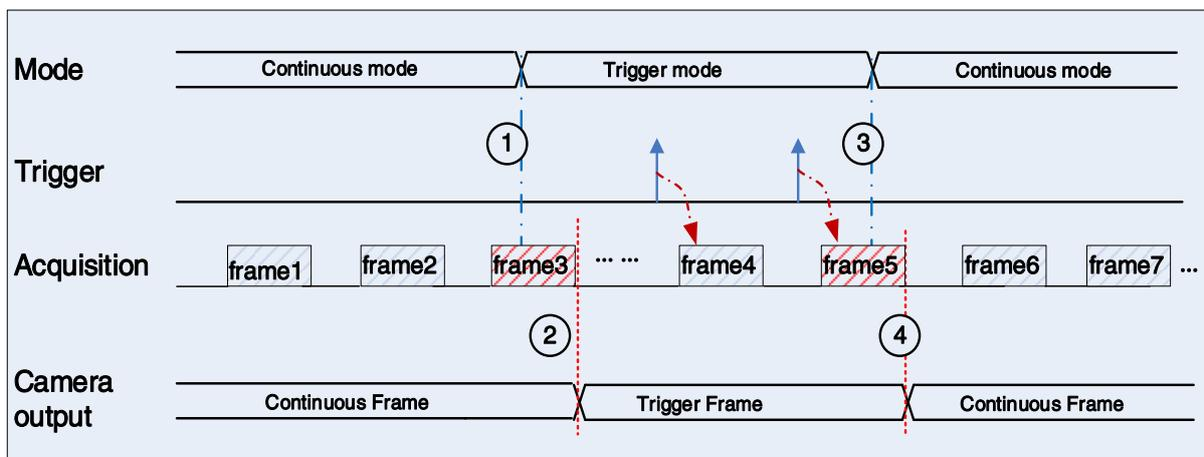
Figure 8-10 Switch trigger mode during frame reading out
