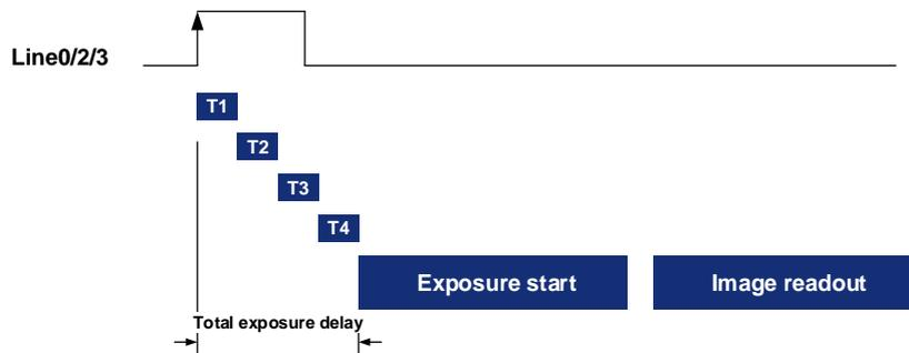
Figure 8-12 Exposure delay
