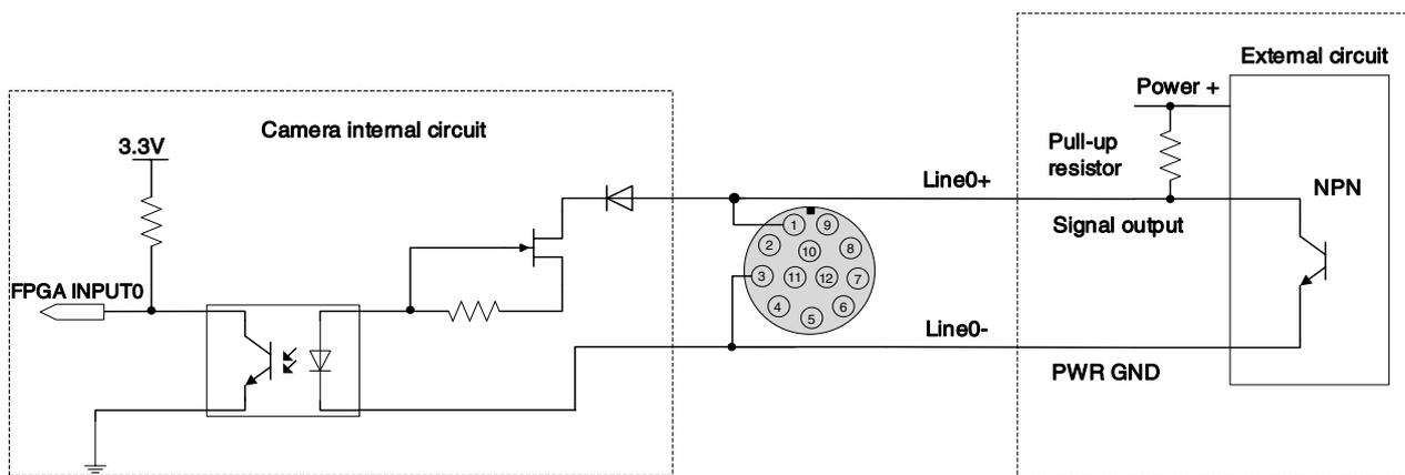
Figure 7-2 NPN photosensor connected to opto-isolated input circuit
