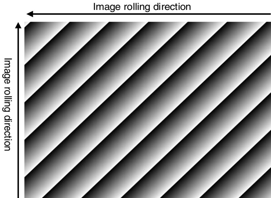
Figure 8-23 Moving diagonal gray gradient test image
