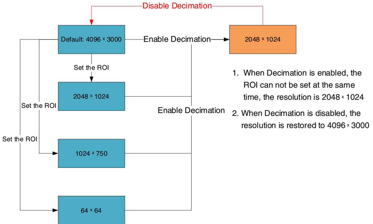
Figure 8-30 Schematic diagram of the relationship between ROI and Decimation
