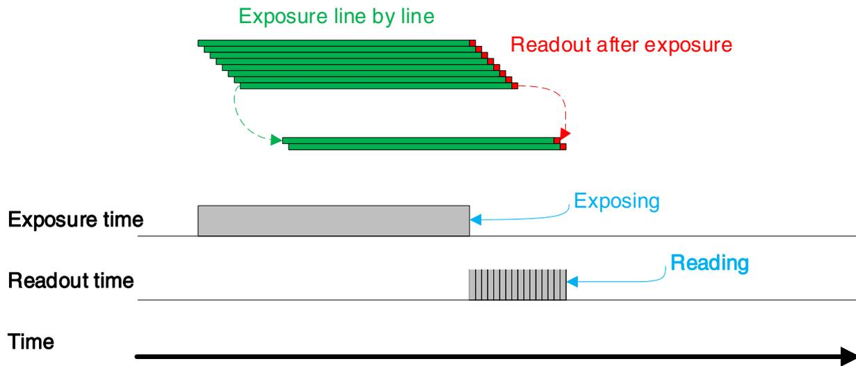
Figure 8-14 Electronic rolling shutter
