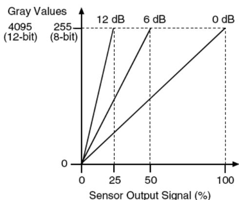
Figure 8-19 The camera's response curve
