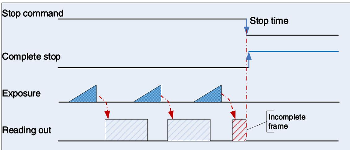
Figure 8-8 Acquisition stop during reading out
