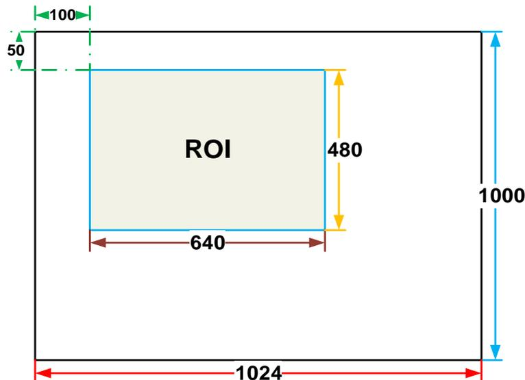
Figure 8-21 An example for the relative position between the ROI and the current image
