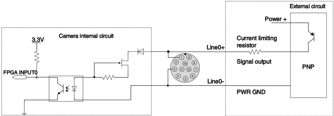
Figure 7-3 PNP photosensor connected to opto-isolated input circuit
