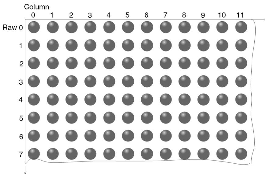
When the pixel format is set to Mono8, the brightness value of each pixel is 8bits. The format in the memory is as follows:
