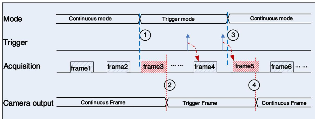
Figure 8-11 Switch trigger mode during blanking (or exposure)
