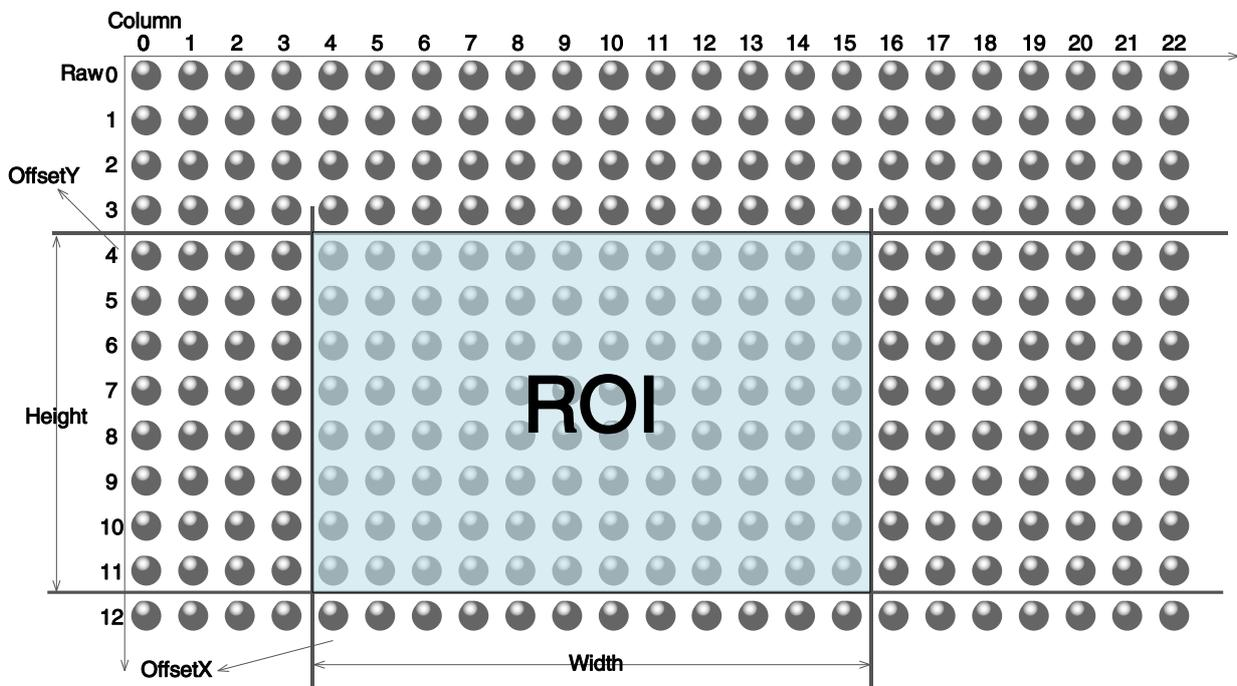
When reducing the height of the ROI, the maximum frame rate of the camera will be raised. Please refer to section 8.5.1 for specific effects on the acquisition frame rate.
