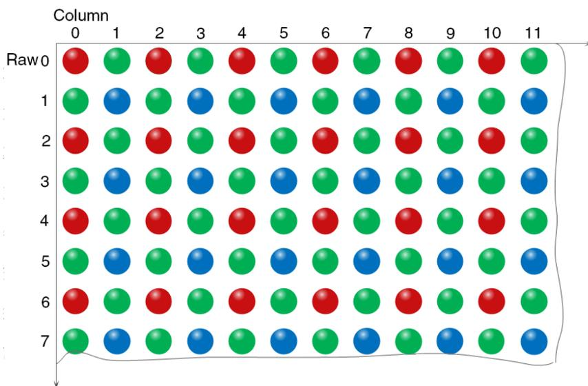
When the pixel format is set to BayerRG8, the value of each pixel in the output image of the camera is 8 bits. According to the location difference, the three components of red, green and blue are respectively represented. The format in the memory is as follows:
