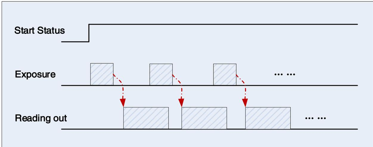
Figure 8-6 Continuous acquisition process
